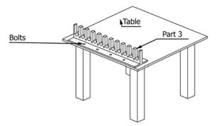
FIG. X1.8 Part 3 Bolted to the Table
