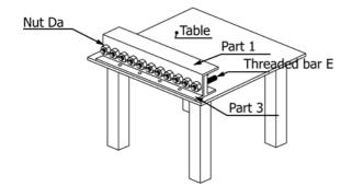
FIG. X1.9 Part 1 Engaged to Part 3, Part 3 Bolted to the Table
