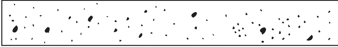
Figure 4-6 Charts for t Over \frac{3}{4} in. to 2 in. (19 mm to 50 mm), Inclusive
