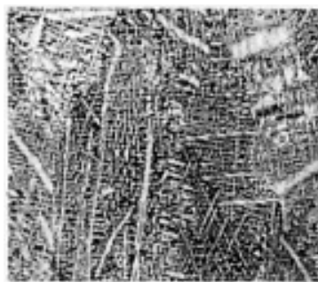
Fig. 31 Copper alloy C71500 (copper nickel, 30%) ingot. Dendritic structure shows coring: light areas are nickel rich; dark areas are low in nickel. 20 \times . Source: 85ASM 13
